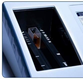
"The Lovibond® Model Fx solves the problem of measuring the colour of edible oils with its unique ability to not only keep the oil at a constant temperature but also to measure and report on the temperature of the sample, avoiding any misreadings from crystallization."
